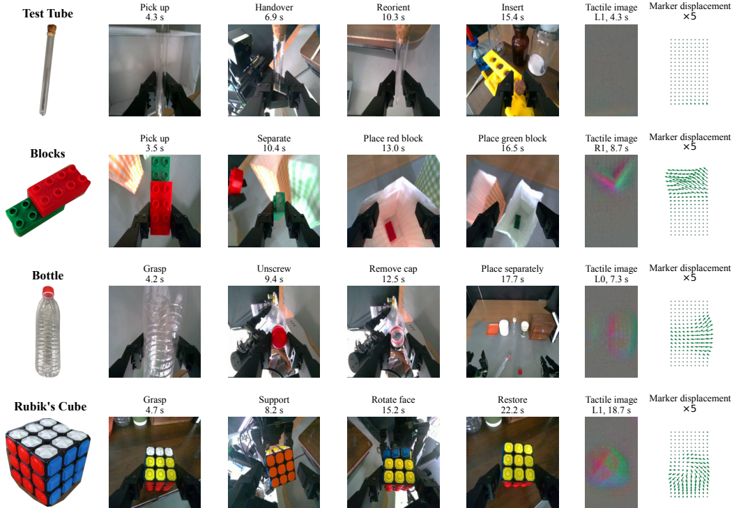
Figure 11: Four bimanual tasks. Object photographs, rollout stages, and paired tactile-image/marker-displacement examples. L/R denotes the gripper and 0/1 its pad; green arrows show recorded displacement at 5\times display scale.
